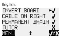
One line of the screen incorporates the *cursor* in the form of a 'blinking' \* sign. By repeatedly pressing  $\hat{v}$  or  $\hat{v}$ , you can move the cursor up and down and view all eleven options in rotation.
