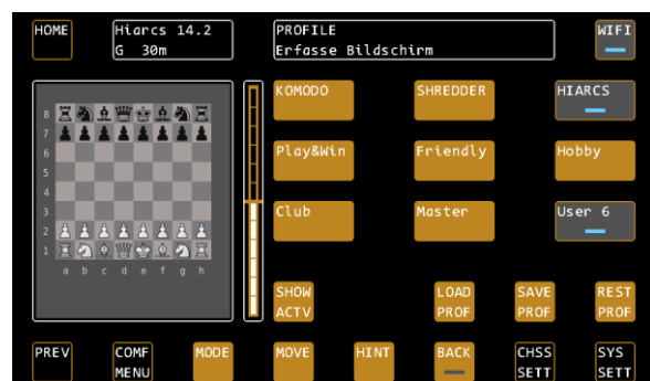
The Hiarc CHAMPION profile has been changed by the user. The modified profile can now be loaded, overwritten (SAVE PROF) or restored (REST PROF).
